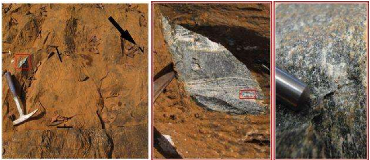
Figure 4-6 Gneissic unit showing foliation and jointing with disseminated sulphides (location: 223043, 1013856 – UTM WGS84 Zone 29N)
