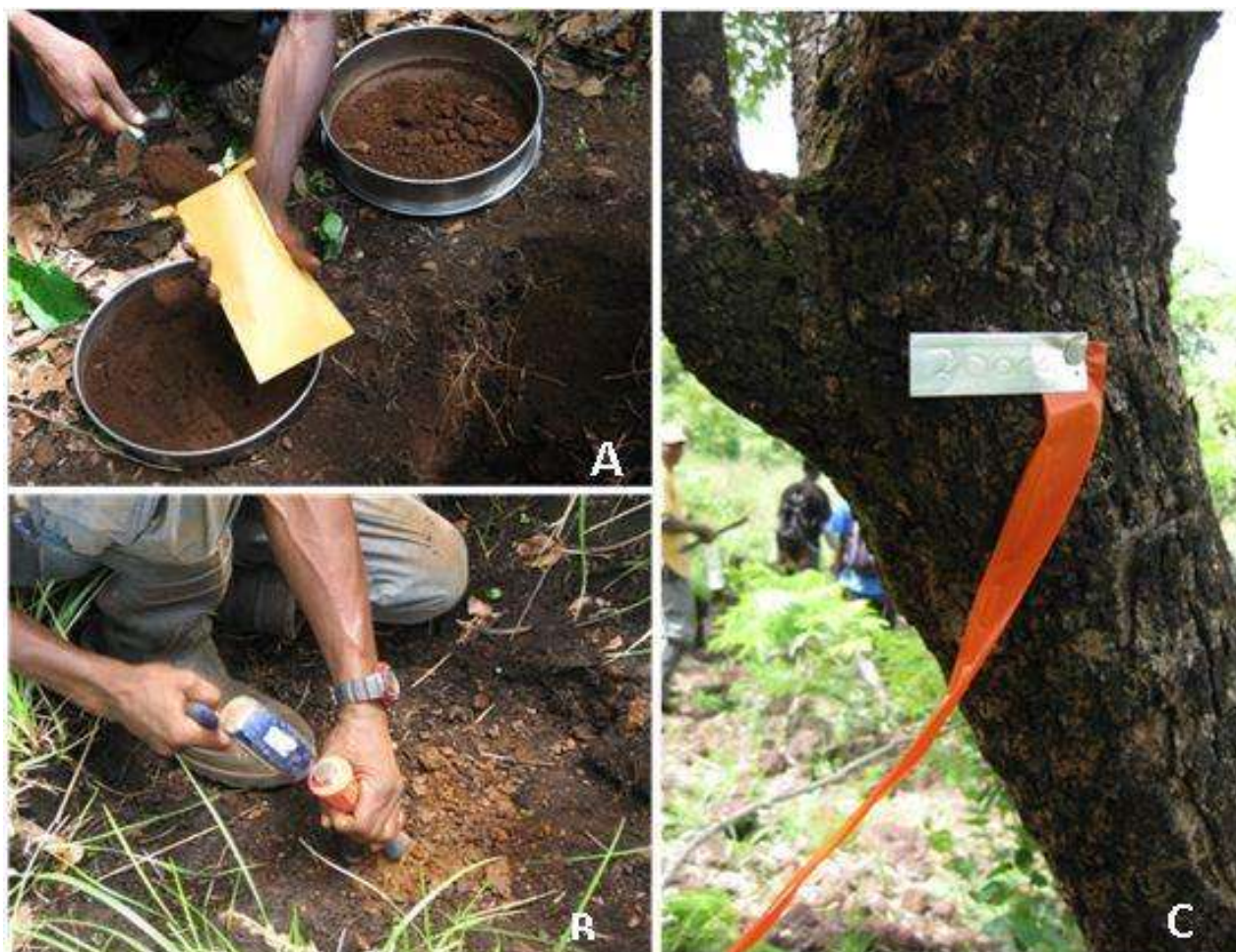
Figure 9-7 Regolith sampling. A – Soil sample from sieved fines. B – Rock chip sample of duricrust. C – Sample tag at sample location.
