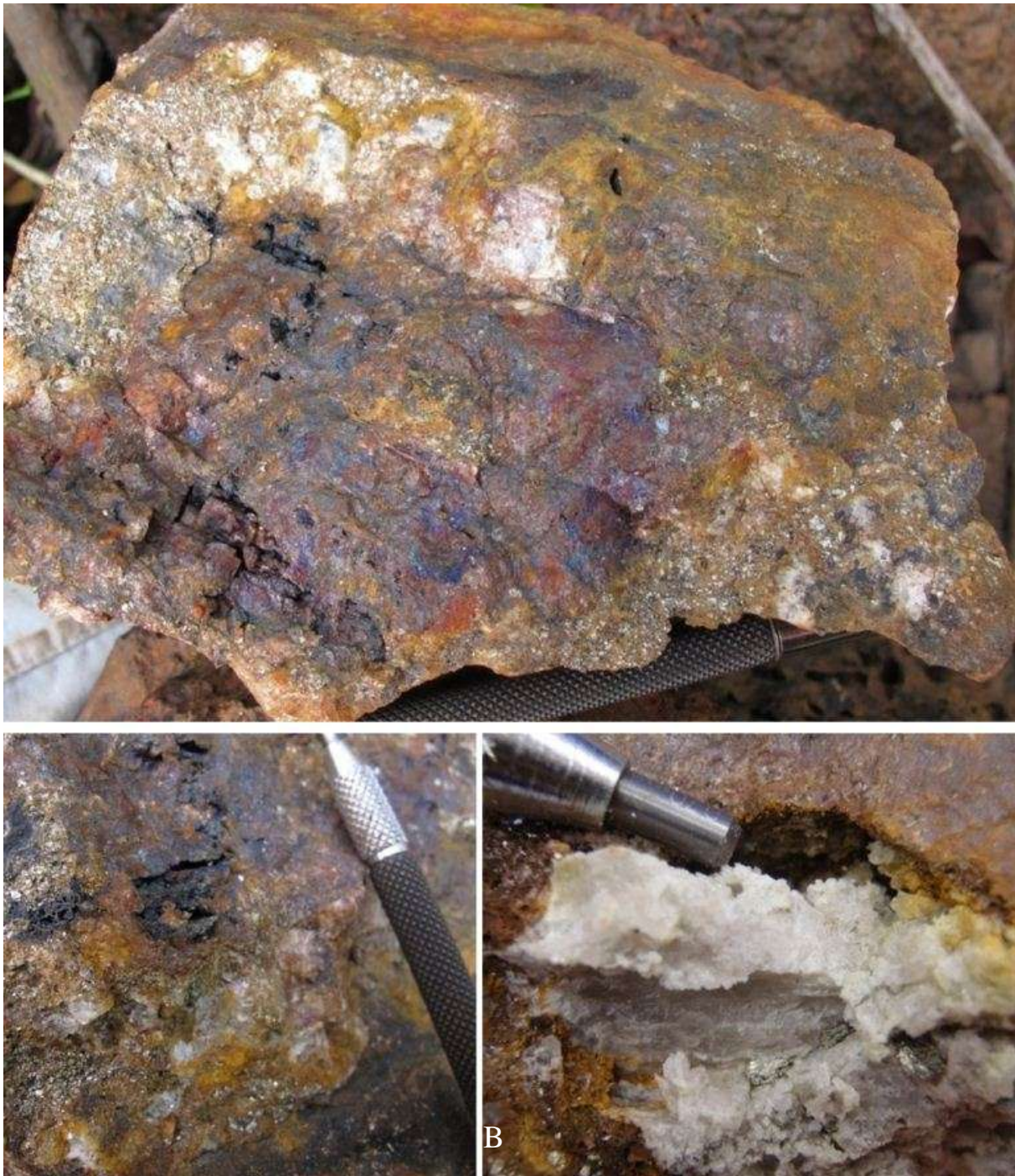
Figure 4-10 Massive mineralised 'Gold Stone'. A – 'Goldstone'. B – Zoomed image showing types of mineralisation. C – Quartz associated with arsenopyrite appears to have filled a void within the laterite/gossan (location 221443, 1017296 – UTM WGS84 Zone 29N).
