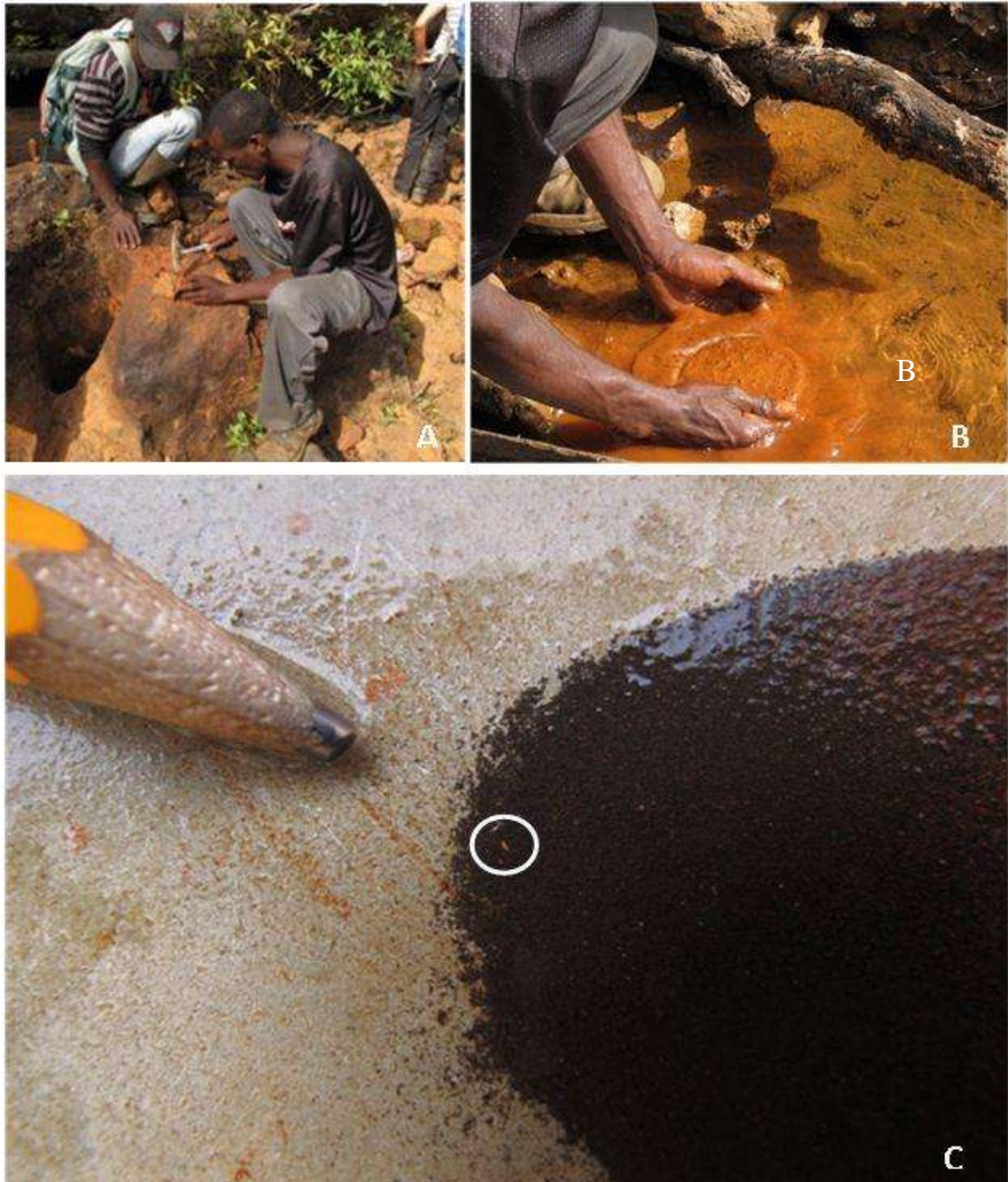
Figure 4-12 Methodology used for gold extraction from 'Gold Stone' occurrences. A – Crushing sample. B – Panning crushed sample. C – Head of tail concentrate showing small gold particle with a flat profile.
