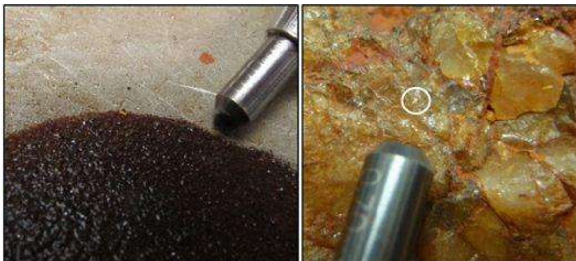
Figure 7-8 Visible Gold from Sample ES0000962: panned fines and gold in quartz
